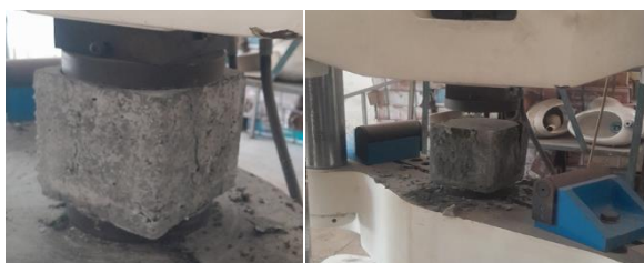
Figure 2. Concrete block testing in UTM machine
