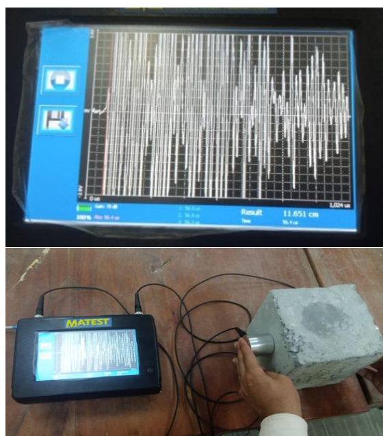
Figure 4. Ultrasonic Pulse Velocity (UPV)
