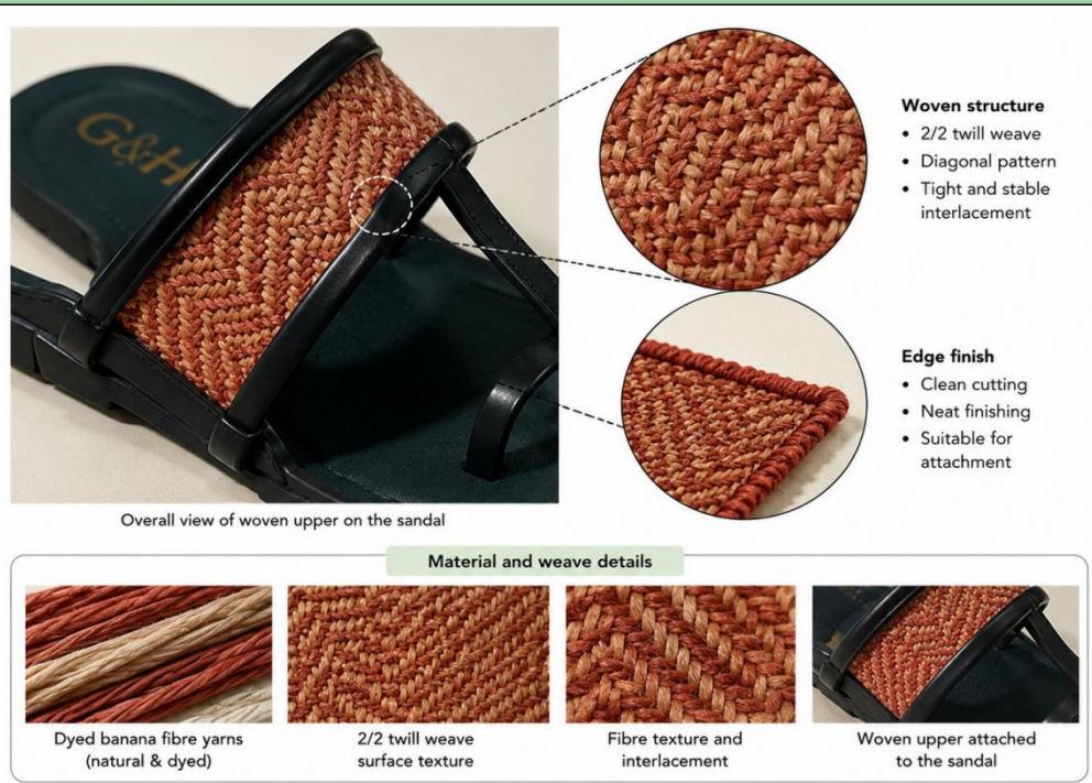
Figure 5. Close-up view of the dyed banana fibre woven upper used in the sandal prototype, showing the 2/2 twill weave structure, texture, and edge finish.
