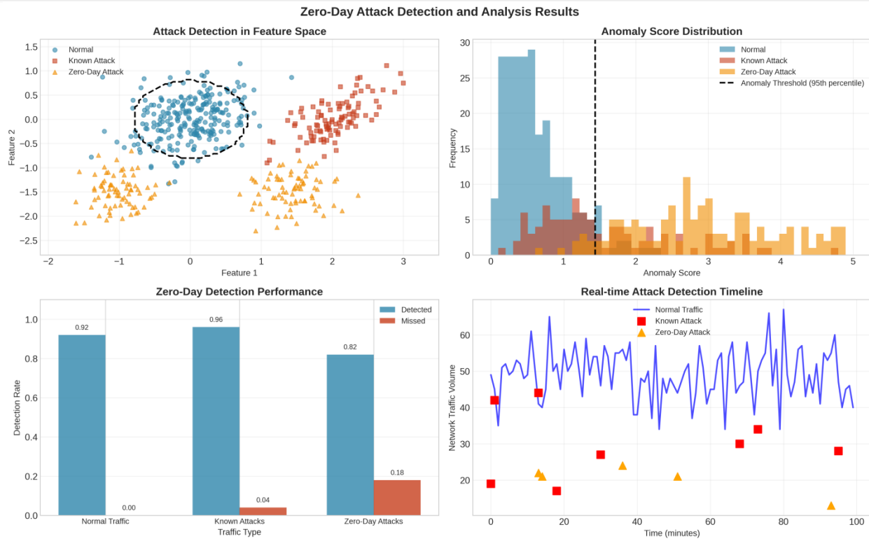
Figure 7. Zero-day attack detection analysis including feature-space separation, anomaly score distribution, detection rates, and real-time attack identification.
