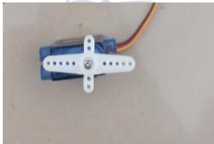
Fig 6. Servo Motor used for locking and unlocking mechanism
