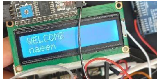
Fig 7. I2C LCD showing access status and user identification messages.
