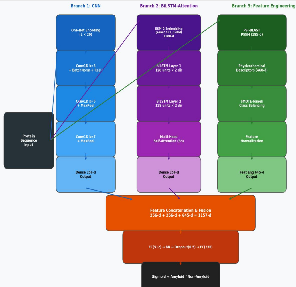
Figure 2: AmyluPred-DL three branches fold over structure. Branch 1 (CNN) can only take on one-hot sequences to detect local motifs. Branch 2 (BiLSTM-Attention) takes ESM-2 long range context. Branch 3 ( Feature Engineering ) works on PSSM +physicochemical descriptors. All branches are recombined (1157-d) and categorized through fully-connected layers of sigmoid output.
