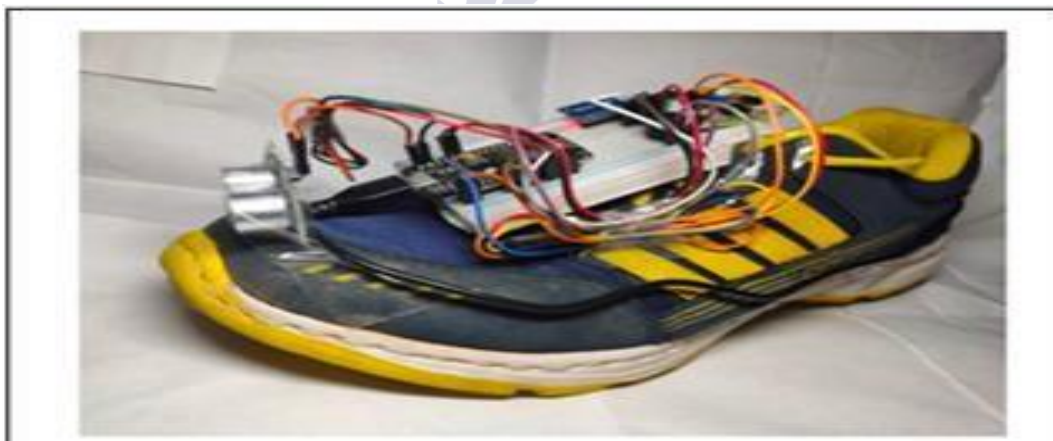
Figure 5: Example of an early assistive-shoe prototype with surface-mounted wiring and external components, illustrating the bulk and discomfort associated with current designs (adapted from Joseph et al., 2023).
