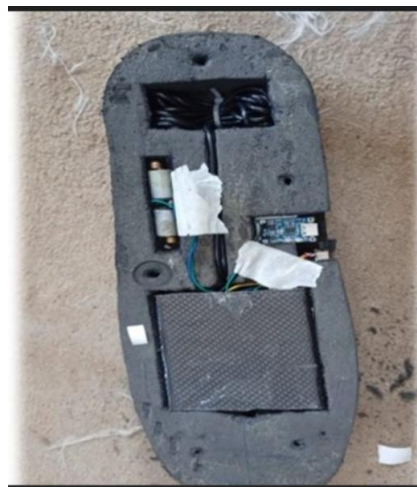
Figure 32: vibration motor placement
