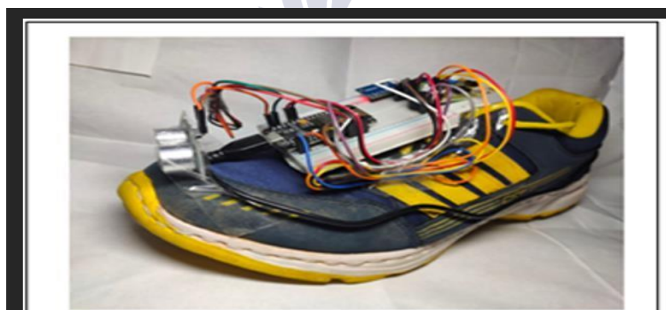
Figure 41: Previous effort electronics mounted externally
