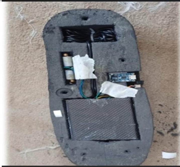
Figure 29: shoe with cavities
