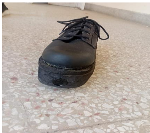
Figure 30: sensor placement in toe region
