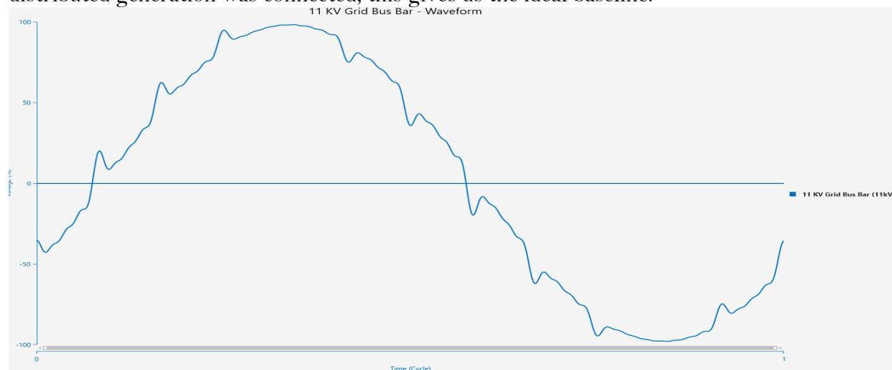
Figure 3: Shows the harmonic analysis on 11 KV Grid Bus Bar (Full DG Integration)
