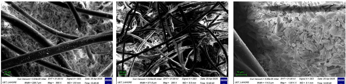
Figure 6 Microstructural analysis of 2.5% recycled textile fiber reinforced gypsum composites
