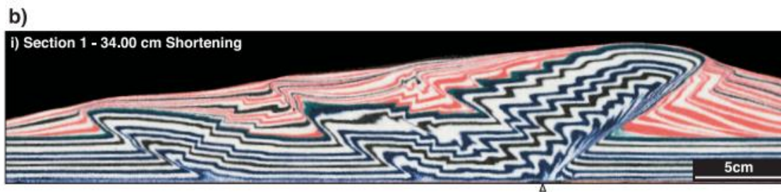
Figure 10: Vertical cross section and line diagram, showing the final geometry of the model. Prowedge thrust faults are marked T1 to T5, in order of nucleation. Note that thrusts T3 and T4 formed out of sequence.
