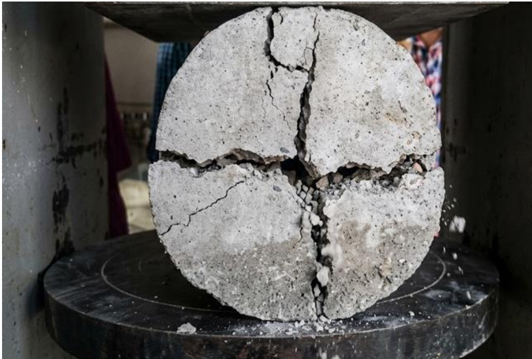
Figure 3. Split tensile test setup with cylinder failure mode for GPC
