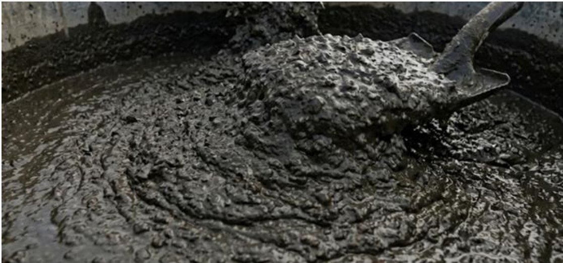
Figure 1. Fresh Geopolymer Concrete
