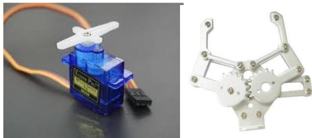
Figure 8: Servo motor with mechanical gripper
