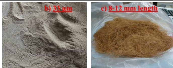
Figure 1: (a) FCBA (Fine coal bottom ash); (b) Coir Fiber
