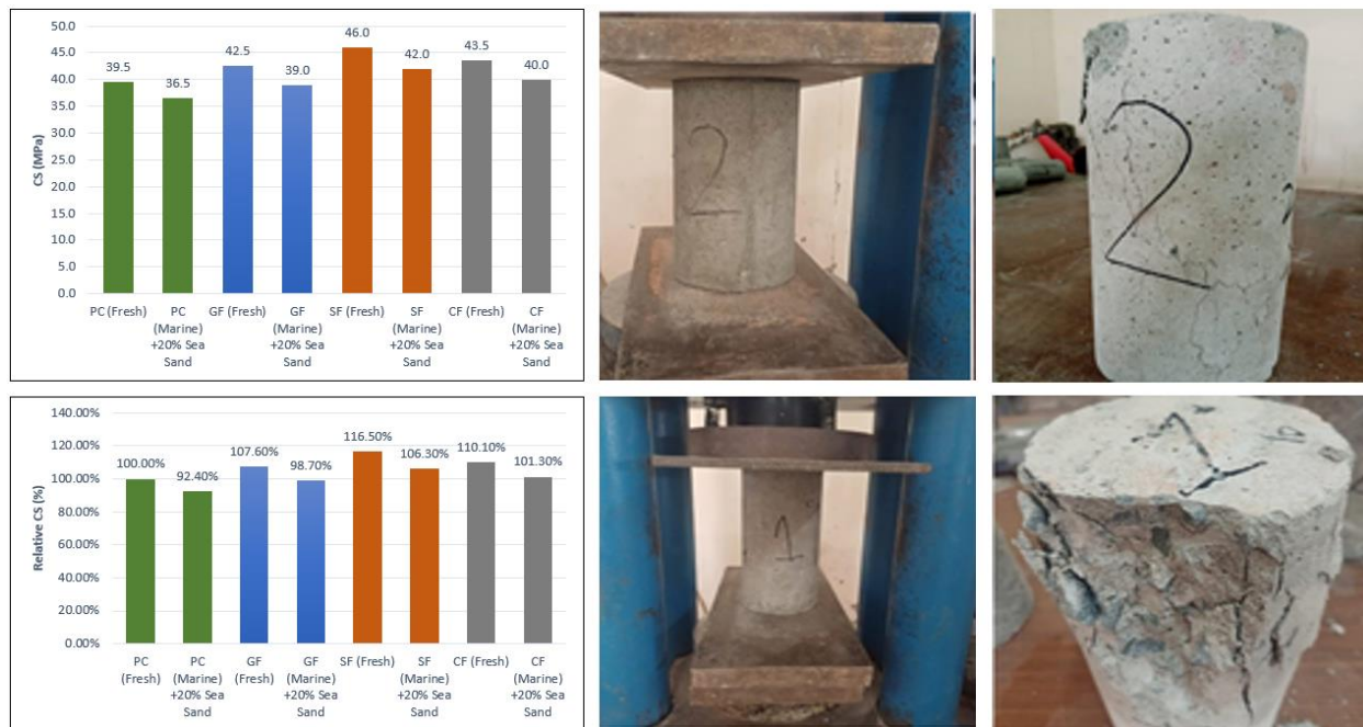
Figure 6: Compressive Strength Samples and Test Results
