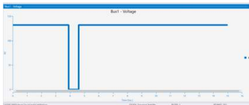
Figure 12: Shows the behavior of bus voltage before, during and, after fault occurrence
