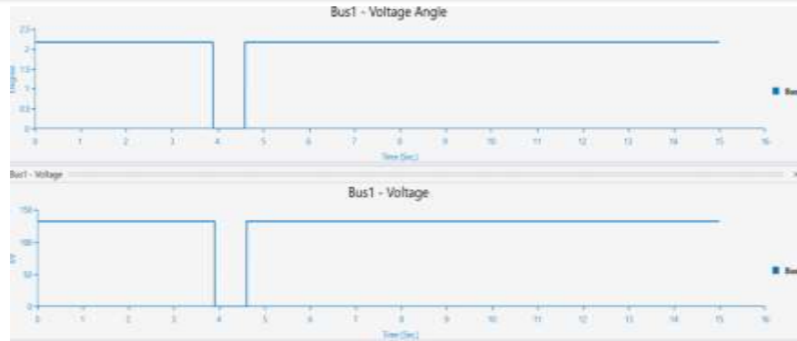
Figure 13: Shows the behavior of bus voltage and voltage angle before, during and, after fault occurrence
