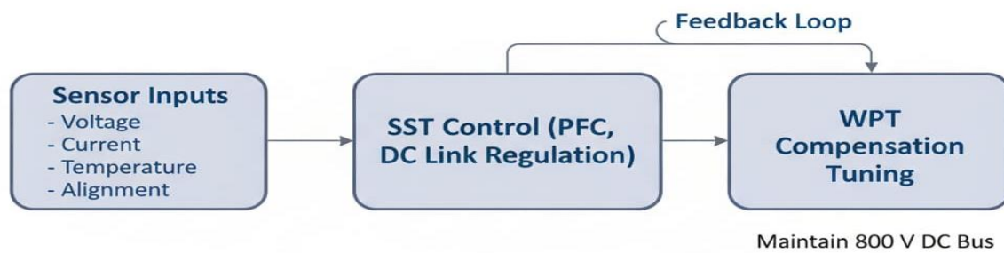
Fig. 3. Adaptive control and feedback workflow of SST + WPT hybrid system, showing sensor inputs and control functions for DC link regulation and WPT tuning.
