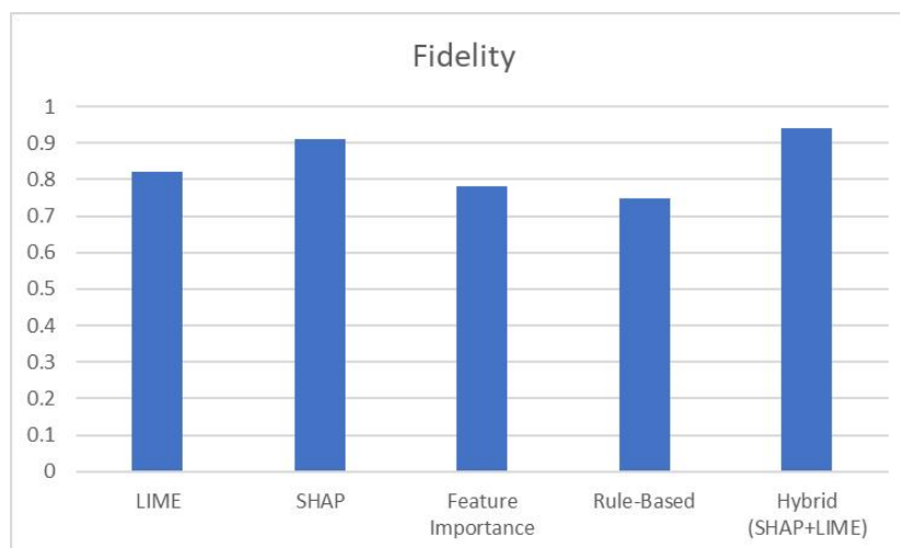
Fig. 3. Comparison of explanation accuracy (fidelity) across different XAI techniques.
