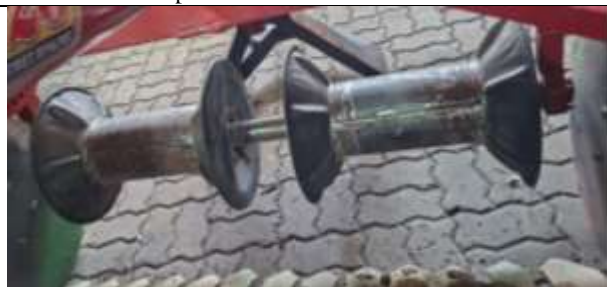
Ridge compaction Drums
