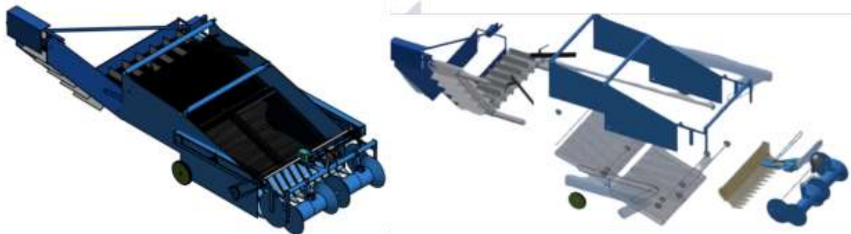
Figure 2. 3D design and explode view of integrated potato digger
