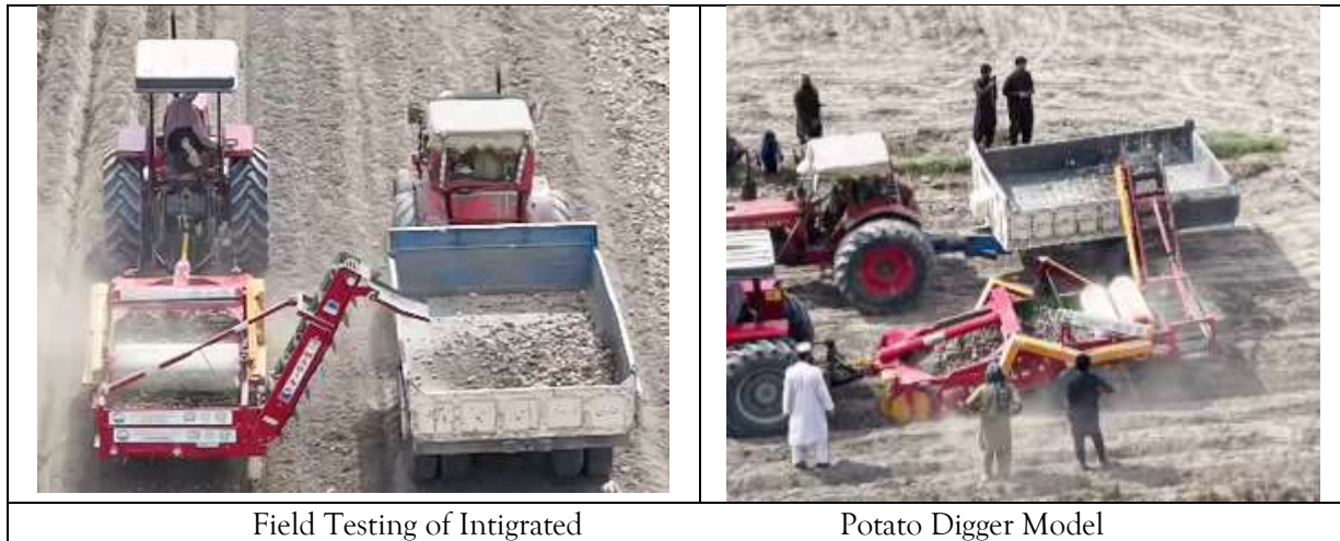
Figure 9. Integrated potato digger components machining processes, assembly and field testing
