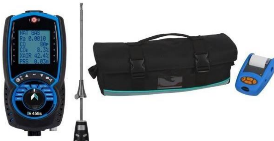
Figure 7. Flue gas analyzer
