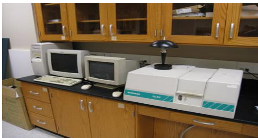
Figure 3.1. UV-Visible spectroscopy setup for measuring optical absorption properties. The technique determines bandgap structure and visible-light absorption efficiency crucial for photocatalytic performance (adapted from Xiaoting et al., 2020).
