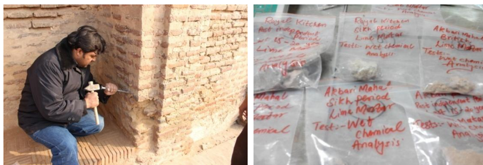
Figure 3 & 4: Extraction of British Period Lime Mortar Specimen in the Left Figure and Packed Specimens in the Right Figure
