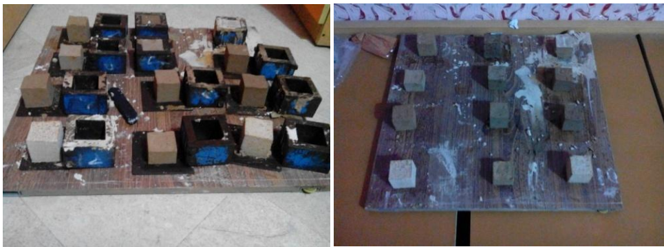
Figure 11 & 12: De-moulding Process in the Left Figure and Air Carbonation Process in the Right Figure
