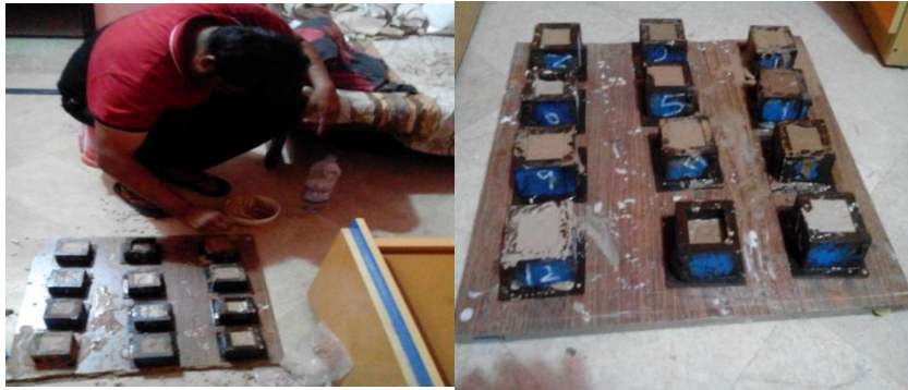
Figure 9 & 10: Moulding Process in the Left Figure and Final Ready moulds in the Right Figure
