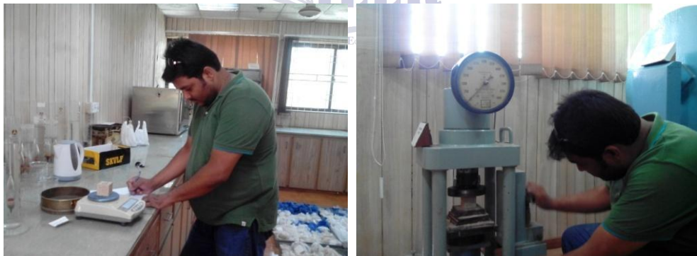
Figure 13 & 14: Weighing Process in the Left Figure and Checking of Crushing Strength in the Right Figure
