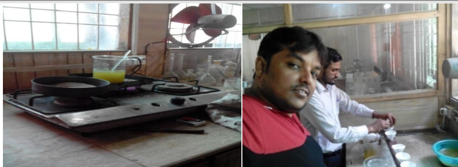
Figure 7 & 8: Wet Chemical Analysis of Lime Mortar Specimen, Heating in the Left Figure and Filtration Process in Right Figure
