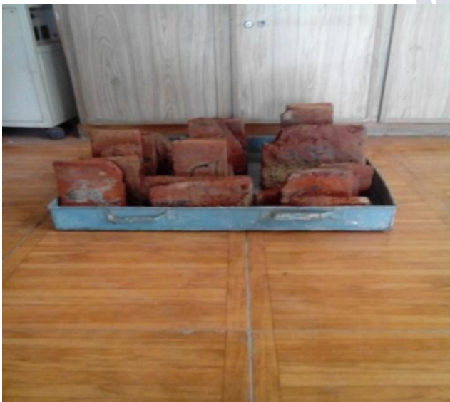
Figure 7&8: Brick Tile Specimens Kept in the Laboratory for Efflorescence Test
