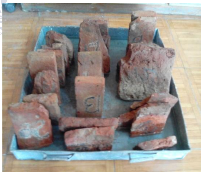
Figure 7&8: Brick Tile Specimens Kept in the Laboratory for Efflorescence Test
