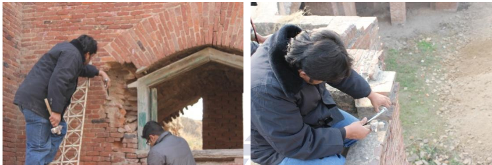
Figure 3 & 4: Extraction of British Period Brick Tile Specimens in the Left Figure and Post-Independence Period in the Right Figure
