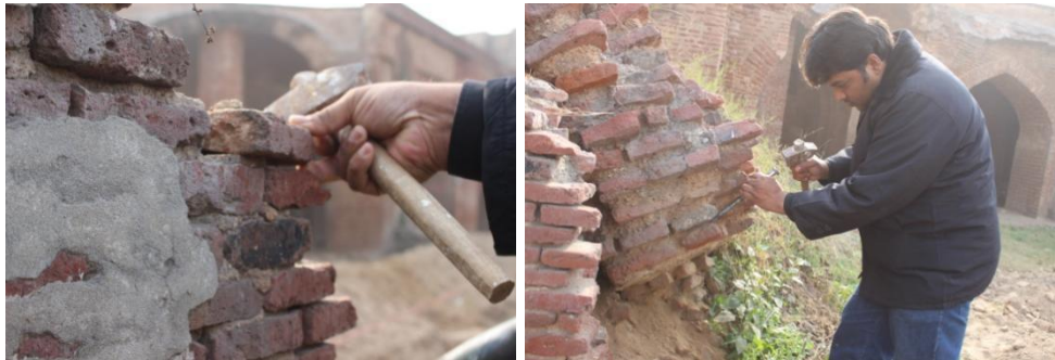
Figure 1 & 2: Extraction of Sikh Period Brick Tile Specimens in the Left Figure and Mughal's Period in the Right Figure
