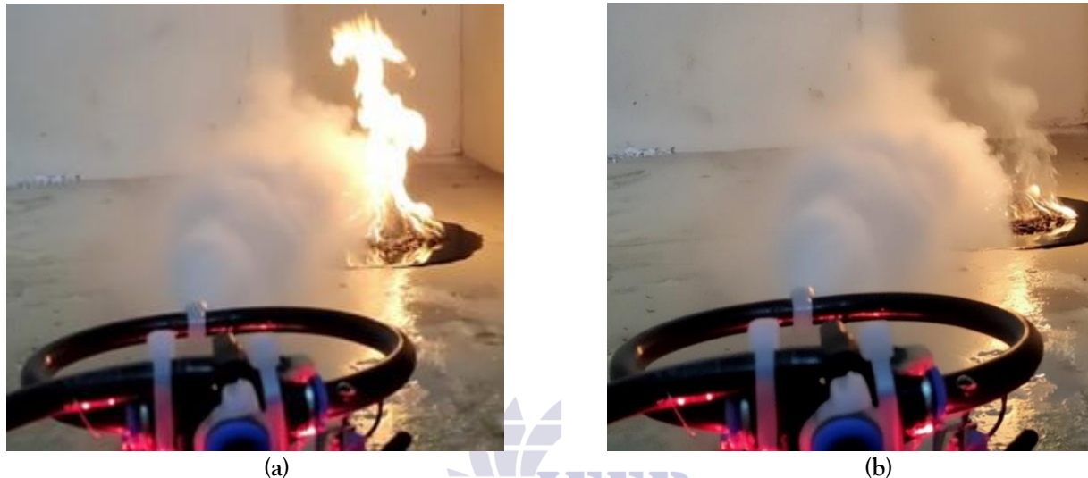
Figure 4. Non-Class A Fire Suppression using CO 2 : (a) CO 2 Discharge during Active Suppression, and (b) Complete Extinguishment after Suppression.
