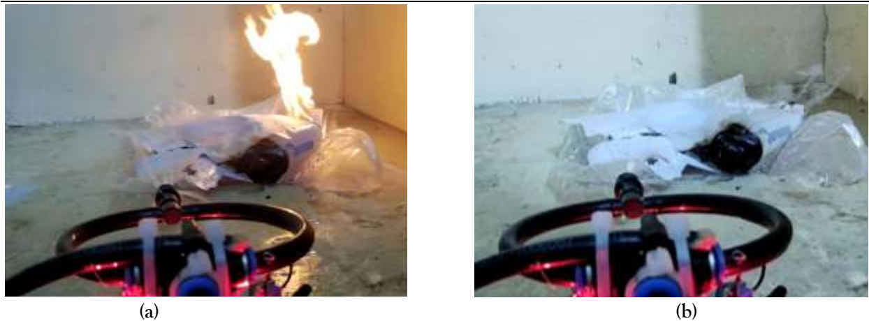
Figure 3. Class A fire Suppression using Water: (a) Water Discharge during Active Suppression, and (b) Complete Extinguishment after Suppression.
