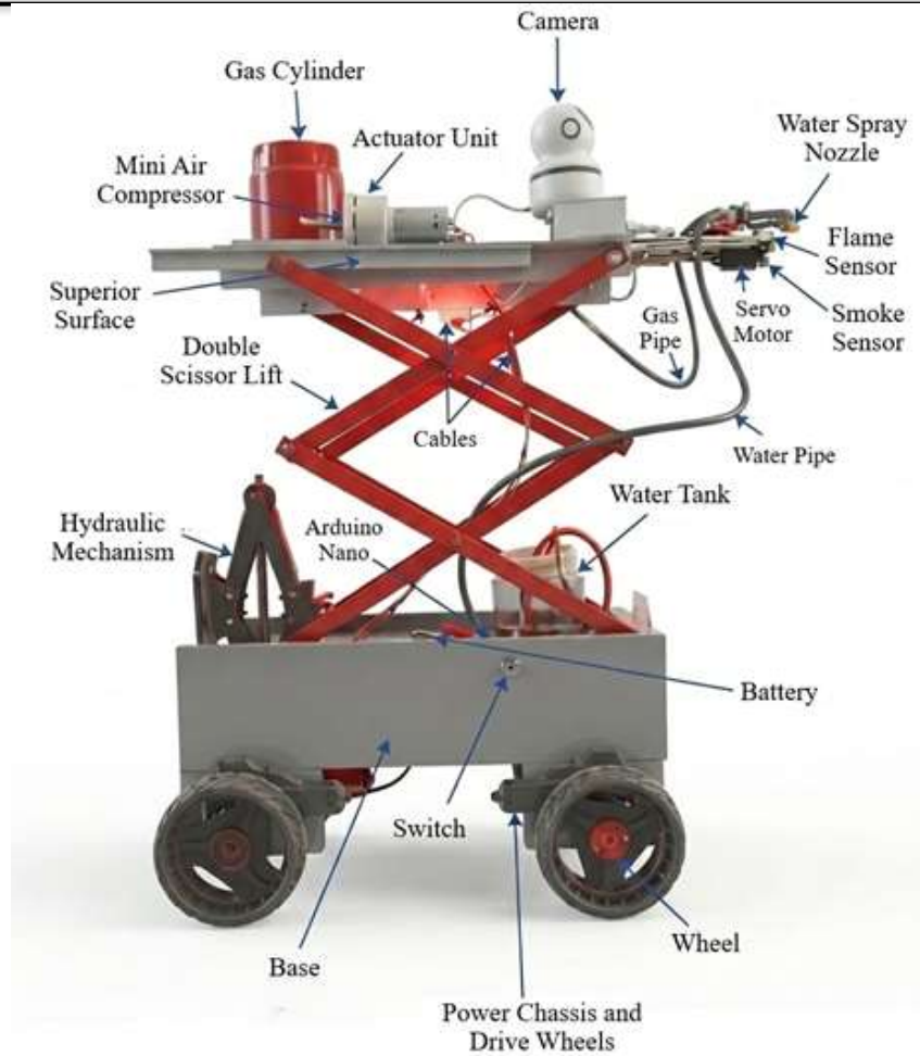
Figure2. Labeled View of the Firefighting Robot Showing all Major Components.
