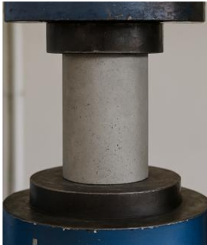
Figure 3. UHPC Cylinders under Compressive Testing.
