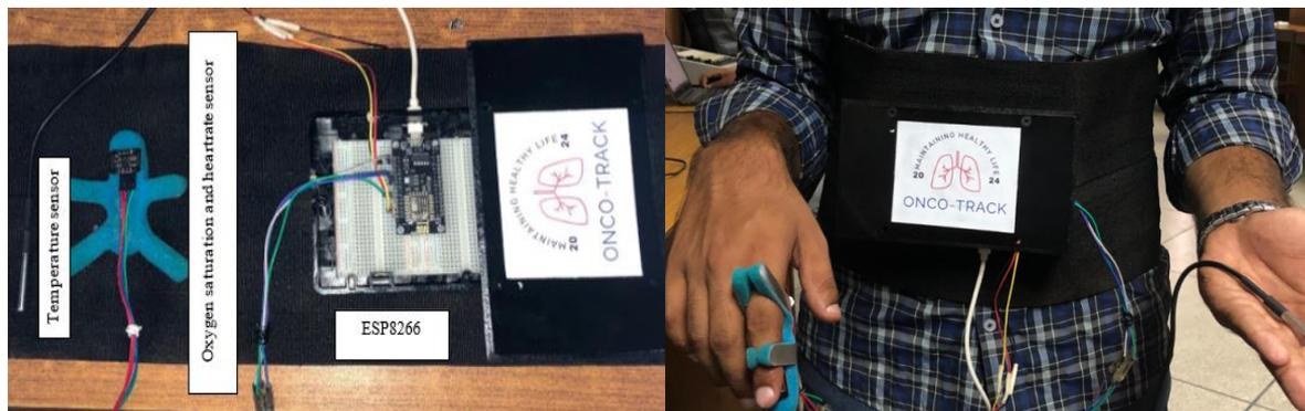
Figure 3-3. Design of all the sensors with ESP8266
