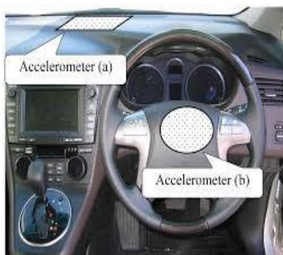
Fig. 15. Location of sensors
