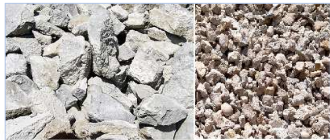
Figure 2: Demolished waste and recycled aggregates
