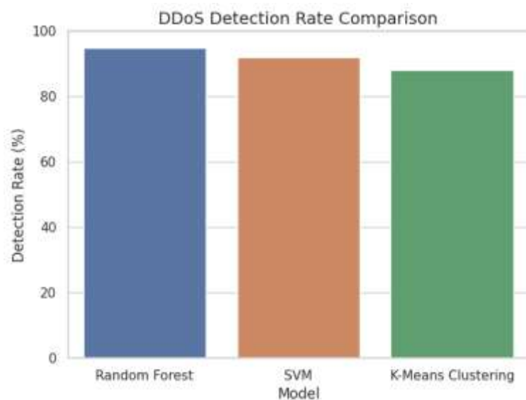
Figure 6: Model Comparison for DDOS Detection Rate
