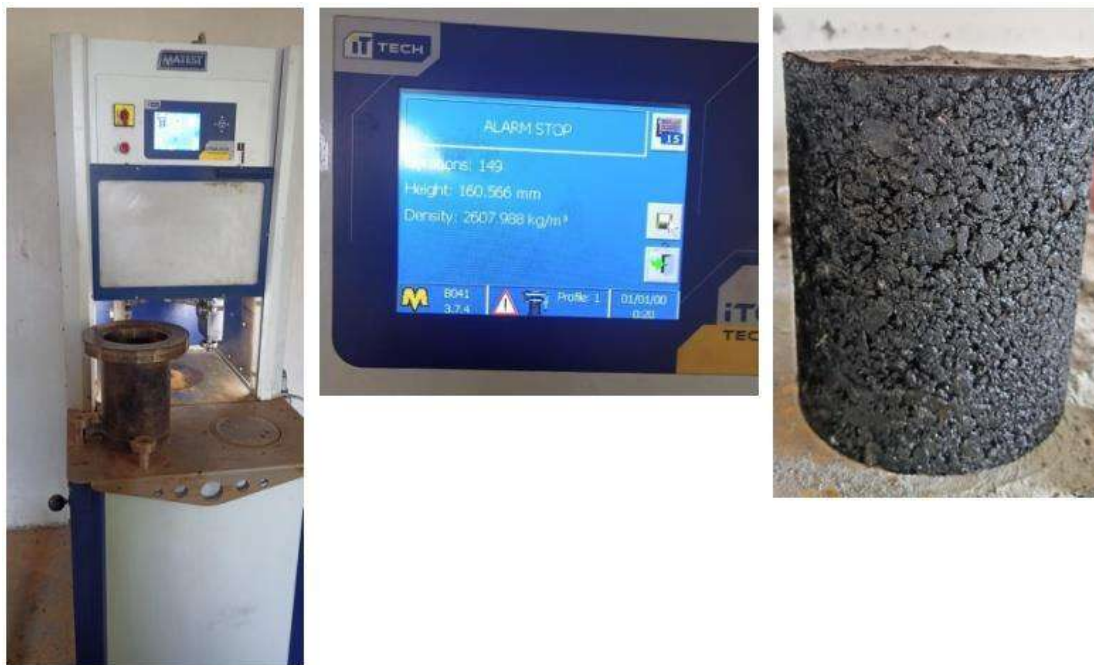
Figure 2. Sample preparation via Superpave Gyratory compactor.
