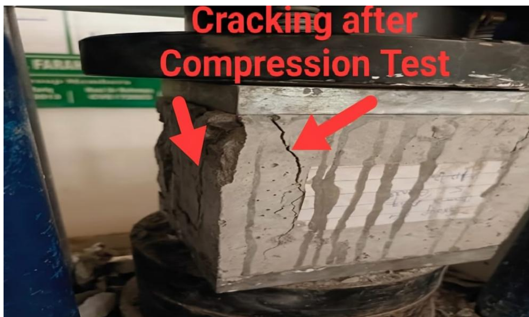
Figure: 9. Compressive Strength of Cubes
