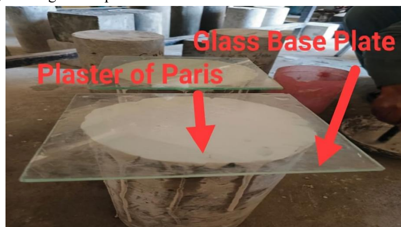
Figure: 8. Capping of Cylinders
